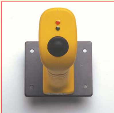
Position 1 (Red LED) STOP Function
