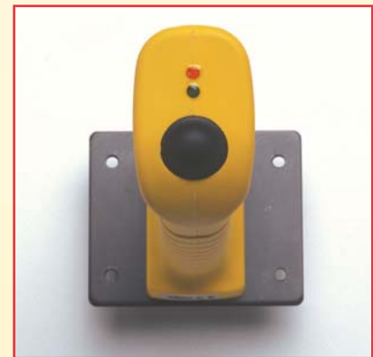
Position 3 (Red LED) STOP Function
